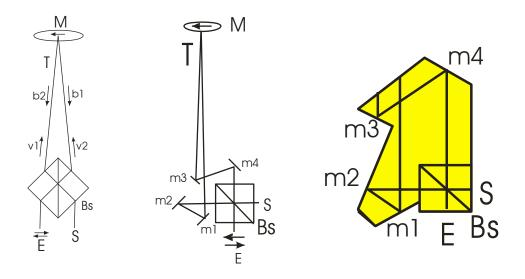
We see below the diagram of the card, next to a preparation of the setup. Notice the mirror m4 in the picture in the middle. We see in it the reflection of the outlined lines on the card. Thus we can adjust by sight as partial. The eye already sees, very accurately whether a mirrored line is in line with the original line. We can see in the reflection that there is still a small error in the adjustment.
