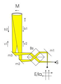
Do we try to widen the lines of interference with this last arrangement. Then look at what shows up. The picture is particularly unstable. Constantly we get a storm of changing interference colors. There is a good explanation for that. We compare it to the basic setup with uneven light path. If the mirror moves there in a minimal way, then the images in E also move, but in the same sense. In a reversal interferometer, of course, the partial beams and the images move in opposite directions.
