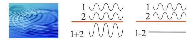
Destructive interference is had when a peak fills a valley. The water then remains at its original level. An analogous phenomenon occurs with light waves, where the merging of a top with a valley leads to darkness.
