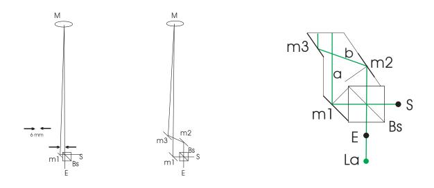
Below is a detail of this setup. We recognize the beamsplitter in the middle, to the right of it the 'point' light source, Below the splitter we see the card and next to it the place for the three flat mirrors that still have to be installed.
