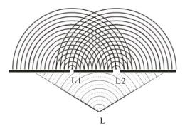
The drawing represents all this in a flat plane. But in reality these are parts of a series of concentric spheres that are constantly expanding and whose waves from one light source are constantly penetrating into another.
