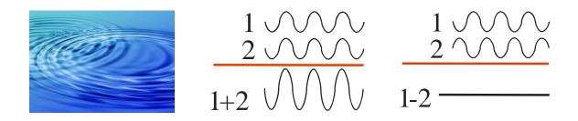
Where two wave tops merge one has a higher top, where two wave valleys merge one obtains a deeper valley. Where a crest fills a valley, the water remains at its original level.
