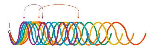
After a few wavelengths, they are quickly "out of sync" with each other so that the distinct colors overlap again. Their colors mix and together give back white light. Interference experiments with white light therefore require greater accuracy than experiment with light of only one color.
