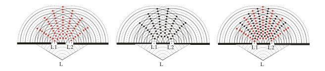
Keep in mind that in reality they are not circles but spheres that keep expanding. Imagine that the black line at the top in the drawing below on the left is a screen we see in top view. Look at it in the drawing in the middle in front view. We see on it the projections of the various lines, as we saw on our wall in the experiment with the large sodium lamp. If we do not work with monochromatic light, but with white light, stripes in interference colors will appear, as shown on the far right.
