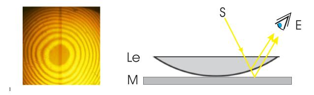
One must imagine that, in fact, numerous light rays across the entire lens surface do this, and that there are light rays reflecting off the underside of the lens that will coincide with other light rays nearby, reflecting off the glass just next to it. Such rays unite and form the various circles of interference.
